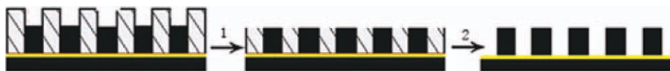
Figure 1 Schematic illustration of the procedures for the post-treatment of the Pth bilayer film. Step 1: mechanical polishing the nanotube surface within AAO template; step 2: removing AAO template and freeze drying. [Color figure can be viewed in the online issue, which is available at wileyonlinelibrary.com .]
